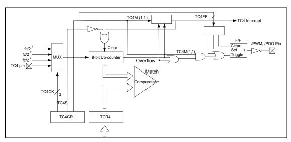
Fig. 5-24 Timer/Counter 4 Configuration
